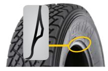
Reinforced sidewall with rim protector ensures that low air pressure will not lead to bead unseating.
